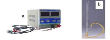
Figure C.2: Electrolysis devices, a) Power Supply, b) Bubble Flow meter
